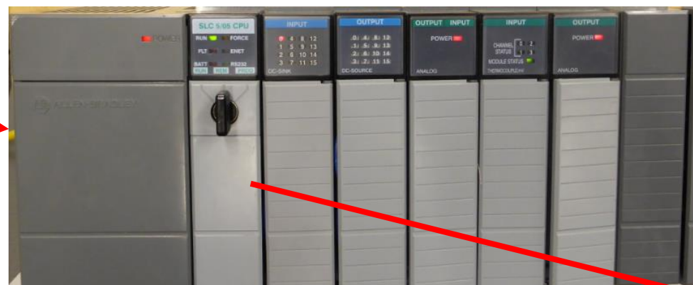
SLC-500 chassis, power supply, processor & I/O modules
