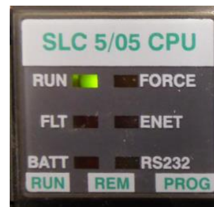
SLC-500 processor diagnostic indicators
